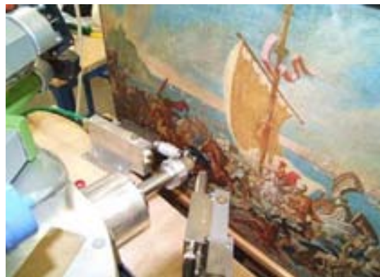
FIGURE 5. The oil in canvas picture being analyzed in the arrangement of the external beam PIXE.
