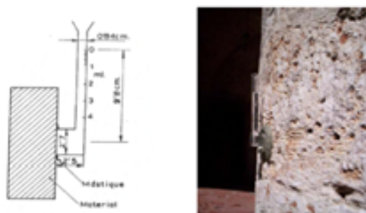
FIGURE 3. “Karsten Pipe” method.
