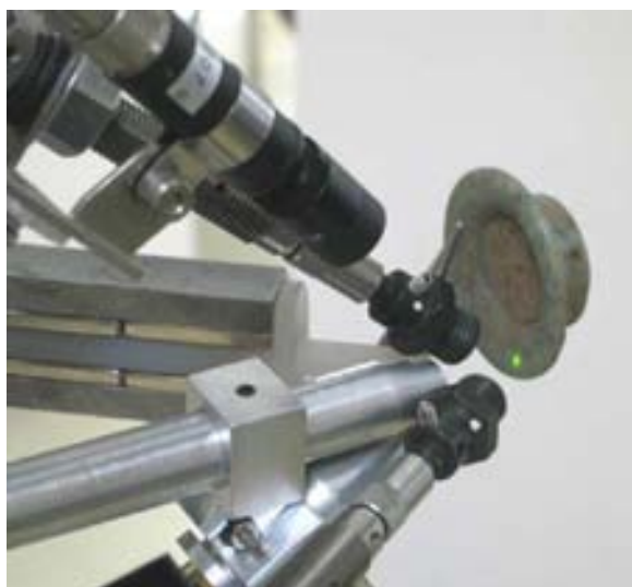
FIGURE 4. External beam setup using two optic spectrometers for a 200 -1000 nm wavelength range. The typical green light emission from jadeite was observed in the ear ornament.
