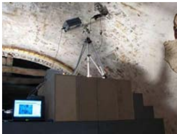
FIGURE 4. The X-ray fluorescence device during the analysis process of wall paintings in their original location.
