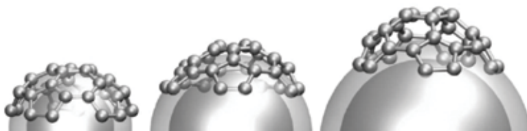
Figure 1: Snapshots showing the simulated lift-off of a graphite cap from a metal nanoparticle undergoing surface fluctuations.
