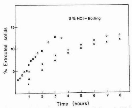
Fig. 1. Percentage of solids in solution as a function of time, for three samples of rice husks boiling in 3% HCl solution.
