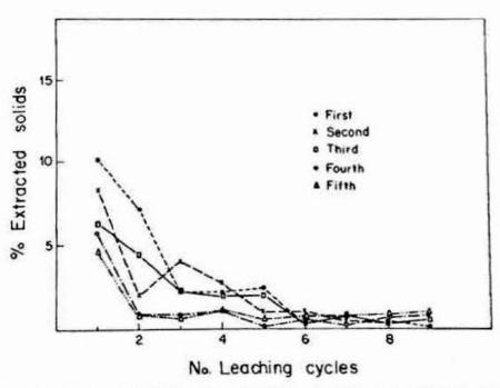
Fig. 3. Percentage of dissolved solids at the end of each leaching process (3% HCl, temperature = 90°C and elapsed time = 6 h), for five different samples of rice husks.
