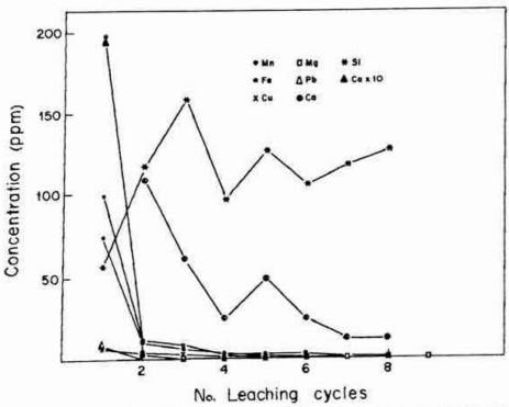
Fig. 4. Concentration of some elements in the 3% HCl solution at the end of each 6 h leaching process at 90°C.
