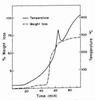
Fig. 5. Weight loss of the leached rice husk, heated in a quartz tube furnace, measuring simultaneously its temperature. The maximum slope in the weight loss corresponds to an exothermic process (burning).
