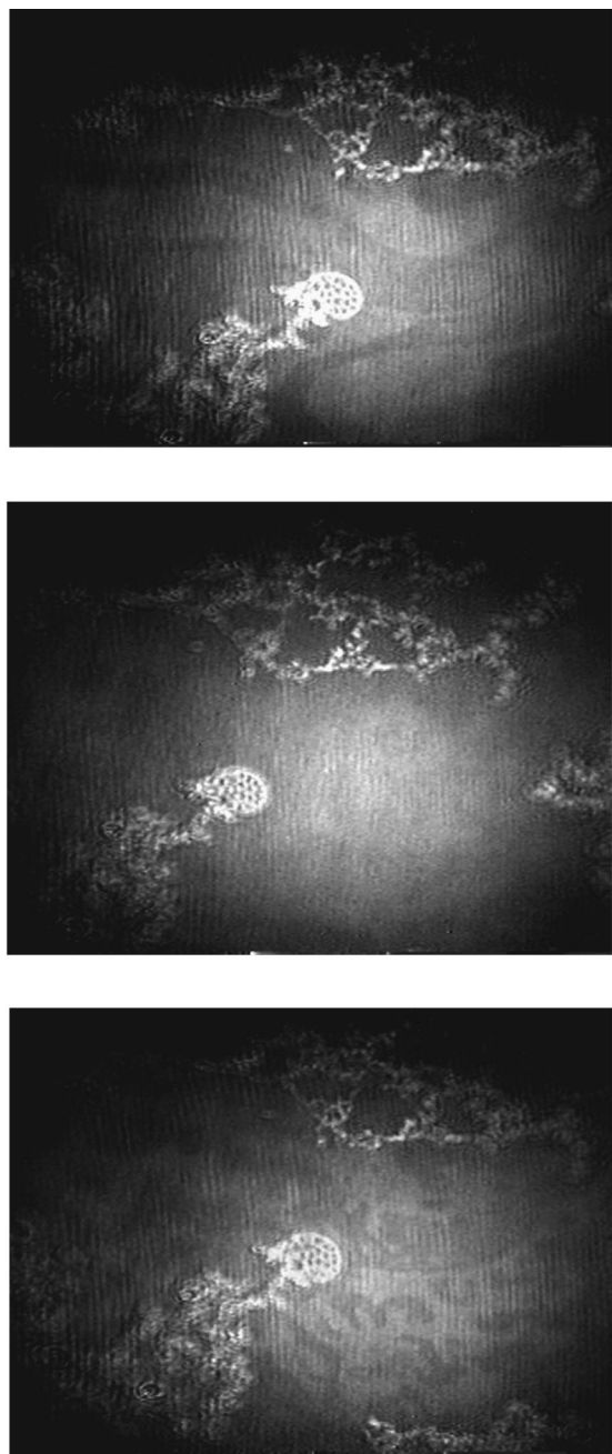
FIG. 4. Phases observed with the BAM in a compression-expansion cycle starting below the Ov - LS phase transition ( T=16.0^\circ\text{C} and \Pi=27.1 - 27.3 mN/m). Ov phase, upper panel; LS phase, medium panel; Ov phase, lower panel.
