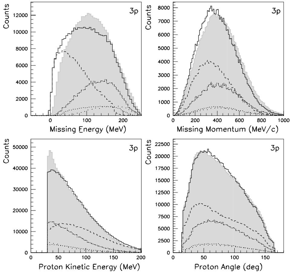
**Fig. 2.** Data from the  $\text{Ar}(\pi^+, 3p)$  reaction at  $T_\pi = 239$  MeV. The shaded areas are the experimental data. The solid lines show how these data are reproduced by the Monte Carlo simulations, with other lines representing individual Monte Carlo components: 3p (dashed), 3p1n (dashed-dotted), 4p (dotted) and 4p1n (wide dotted).
