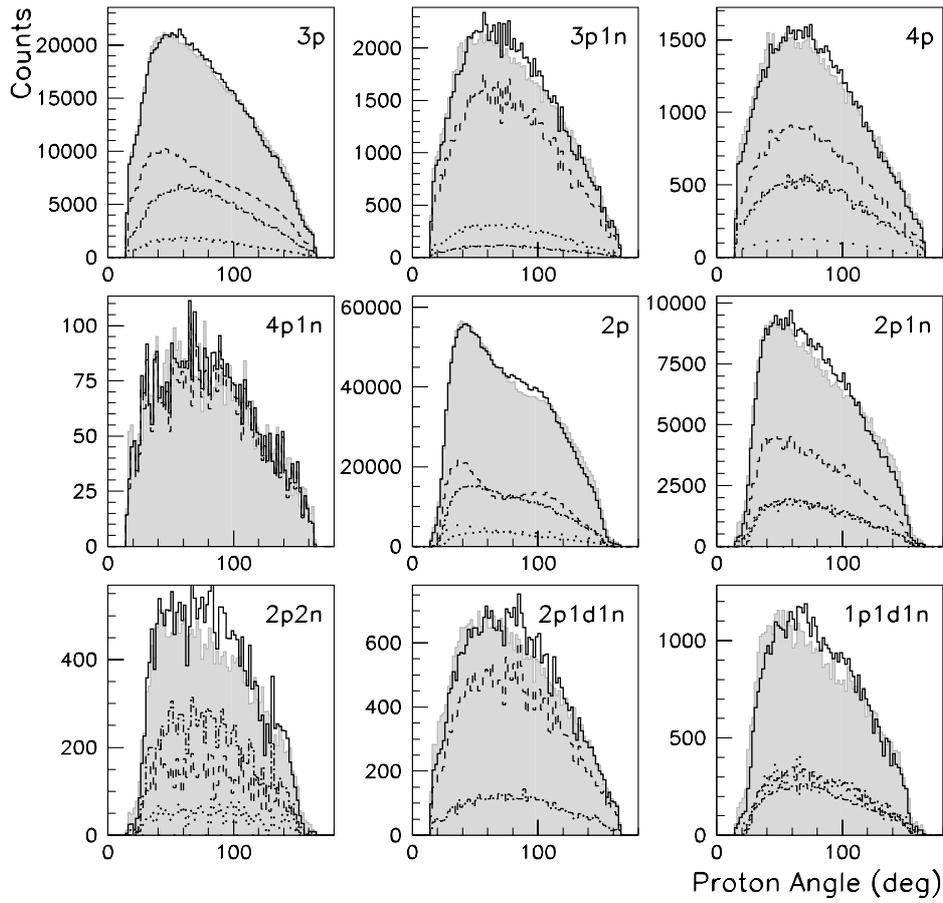
**Fig. 5.** Proton polar-angle distributions for selected channels following the  $\pi^+$  + Ar pion absorption reaction at  $T_\pi = 239$  MeV. The shaded areas are the experimental data. The solid lines show how these data are reproduced by the Monte Carlo simulations. All other lines (dashed, dotted, wide-dotted and dashed-dotted) represent dominant components of the Monte Carlo fit.
