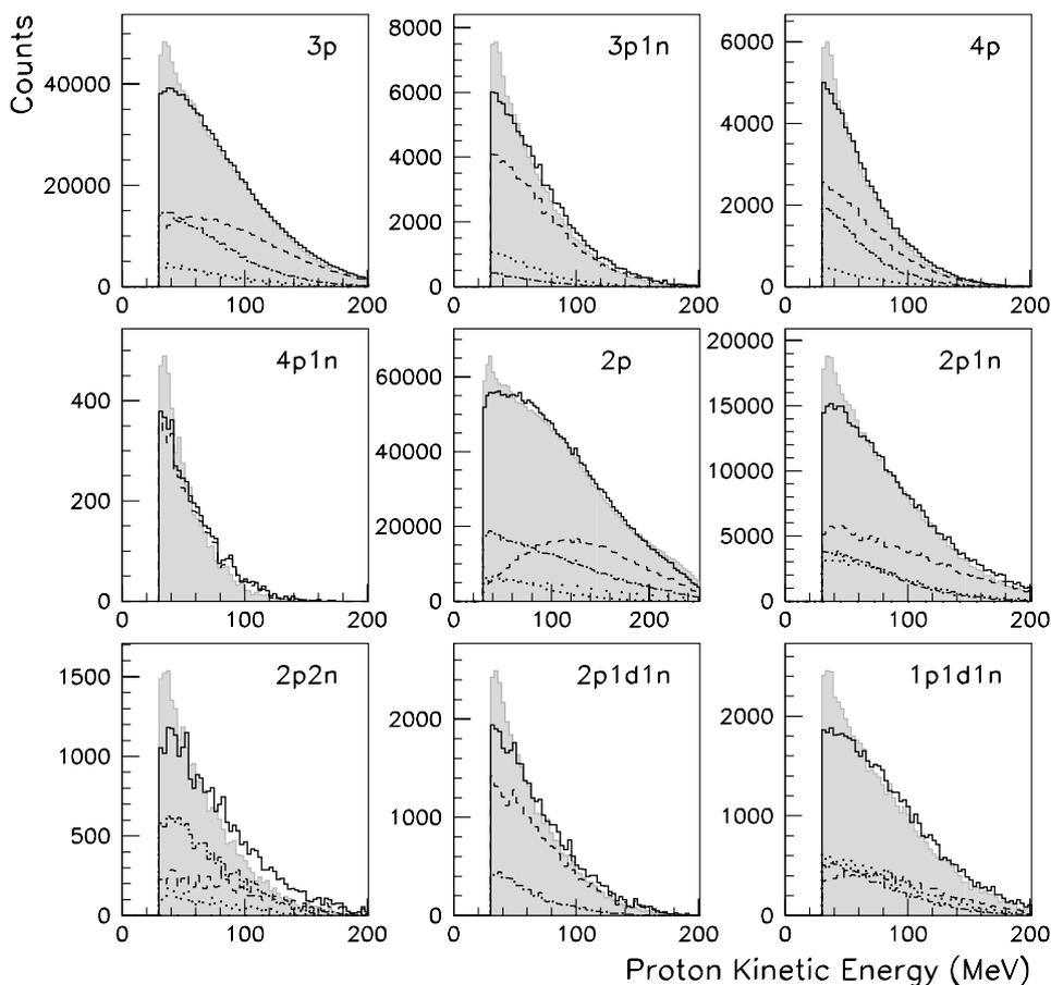
**Fig. 6.** Proton kinetic-energy distributions for selected channels following the  $\pi^+$  + Ar pion absorption reaction at  $T_\pi = 239$  MeV. The shaded areas are the experimental data. The solid lines show how these data are reproduced by the Monte Carlo simulations. All other lines (dashed, dotted, wide-dotted and dashed-dotted) represent dominant components of the Monte Carlo fit.
