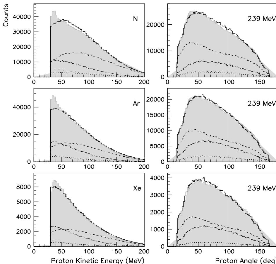
**Fig. 4.** Polar-angle and kinetic-energy distributions for the protons from the  $(\pi^+, 3p)$  reaction on N, Ar and Xe targets at  $T_\pi = 239$  MeV. The shaded areas are the experimental data. The solid lines show how these data are reproduced by the Monte Carlo simulations. The meaning of other lines is as in fig. 2.
