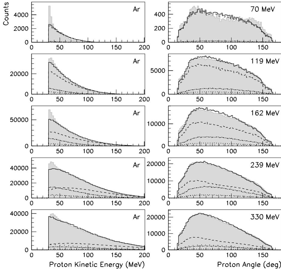
**Fig. 3.** Polar-angle and kinetic-energy distributions for the protons from the  $\text{Ar}(\pi^+, 3p)$  reaction at five pion energies. The shaded areas are the experimental data. The solid lines show how these data are reproduced by the Monte Carlo simulations. The meaning of the other lines is as in fig. 2.
