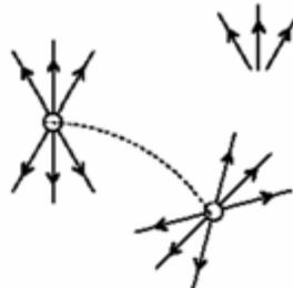
In a light source electrons follow curved trajectories in bend magnets and insertion devices. The transverse acceleration creates  $e^- - \gamma$  separation generating **synchrotron radiation**.
