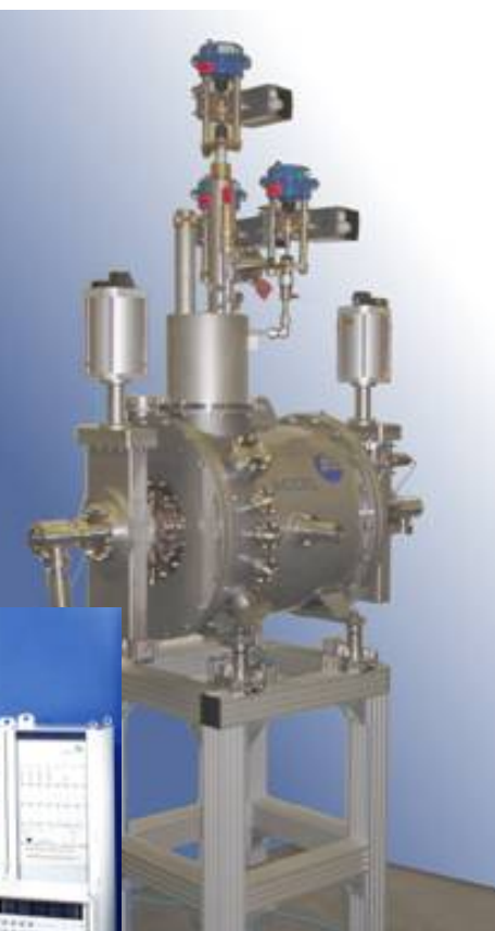
3rd harmonic, 1500 MHz Landau Module for BESSY (Inhouse Development)
