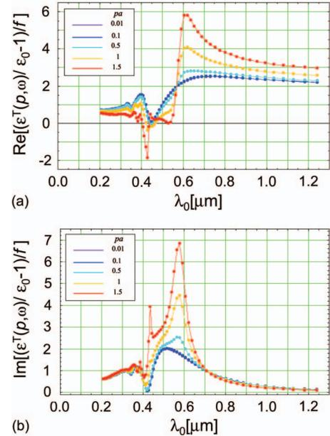
FIG. 8. (Color) Contribution of titanium-dioxide particles to the transverse component of the nonlocal dielectric function [(a) real and (b) imaginary part], normalized to the volume filling fraction, for several values of  $pa$ , as a function of the vacuum wavelength  $\lambda_0$ . The particle radius is fixed at  $a=0.1 \mu\text{m}$ .
