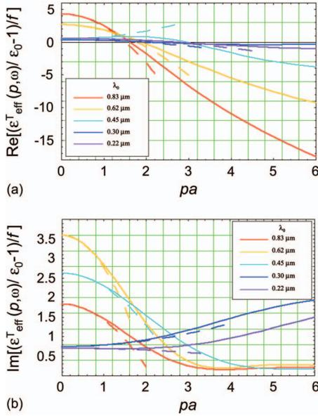
FIG. 2. (Color) Contribution of silver particles to the transverse component of the nonlocal dielectric function [(a) real and (b) imaginary part], normalized to the volume filling fraction, as a function of  $pa$ , for several vacuum wavelengths. The particle radius is fixed at  $a=0.1 \mu\text{m}$ .
