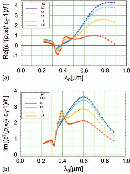
FIG. 6. (Color) Contribution of silver particles to the transverse component of the nonlocal dielectric function [(a) real and (b) imaginary part], normalized to the volume filling fraction, for several values of  $pa$ , as a function of the vacuum wavelength  $\lambda_0$ . The particle radius is fixed at  $a=0.1 \mu\text{m}$ .
