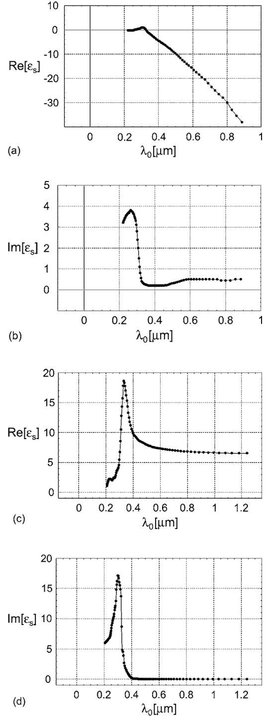
FIG. 1. Experimental data of the real and imaginary parts of the index of refraction for silver and titanium dioxide as a function of frequency or wavelength in vacuum. (a) Real and (b) imaginary part for silver and, (c) real and (d) imaginary part for titanium dioxide.
