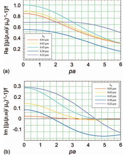
FIG. 12. (Color) Real (a) and imaginary (b) parts of the inverse of the effective nonlocal magnetic permeability minus one, normalized to the volume filling fraction  $f$ , as a function of  $pa$ , for different vacuum wavelengths. The colloidal system is made of silver particles and with radius set at  $a=0.1 \mu\text{m}$ .
