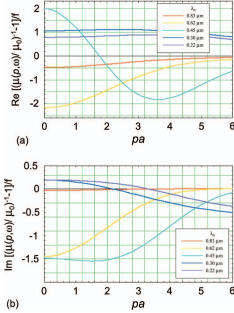
FIG. 13. (Color) Real (a) and imaginary (b) parts of the inverse of the effective nonlocal magnetic permeability minus one, normalized to the volume filling fraction  $f$ , as a function of  $pa$ , for different vacuum wavelengths. The colloidal system is made of titanium-dioxide particles and with radius set at  $a=0.1 \mu\text{m}$ .
