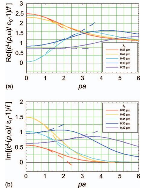
FIG. 5. (Color) Contribution of titanium-dioxide particles to the longitudinal component of the nonlocal dielectric function [(a) real and (b) imaginary part], normalized to the volume filling fraction, as a function of  $pa$ , for several vacuum wavelengths. The particle radius is fixed at  $a=0.1 \mu\text{m}$ .
