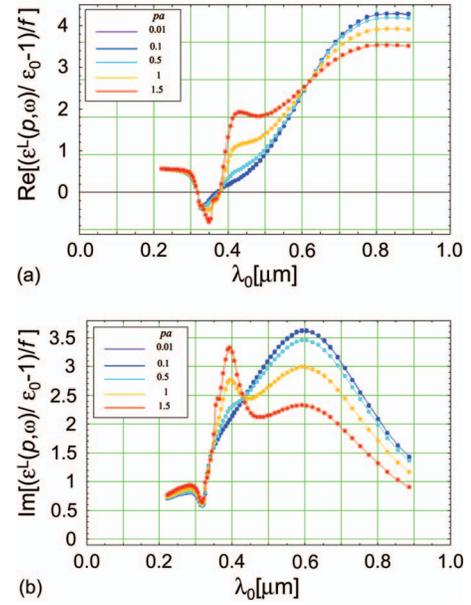
FIG. 7. (Color) Contribution of silver particles to the longitudinal component of the nonlocal dielectric function [(a) real and (b) imaginary part], normalized to the volume filling fraction, for several values of  $pa$ , as a function of the vacuum wavelength  $\lambda_0$ . The particle radius is fixed at  $a=0.1 \mu\text{m}$ .
