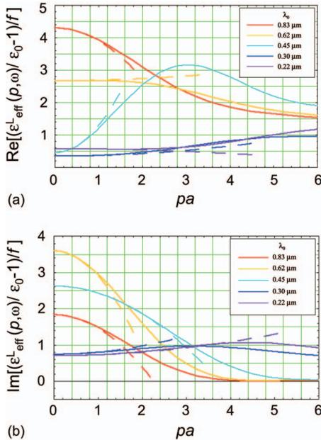
FIG. 3. (Color) Contribution of silver particles to the longitudinal component of the nonlocal dielectric function [(a) real and (b) imaginary part], normalized to the volume filling fraction, as a function of  $pa$ , for several vacuum wavelengths. The particle radius is fixed at  $a=0.1 \mu\text{m}$ .
