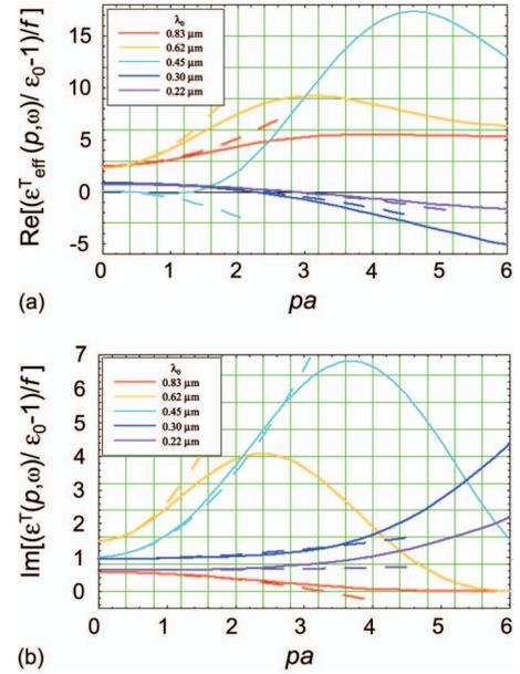
FIG. 4. (Color) Contribution of titanium-dioxide particles to the transverse component of the nonlocal dielectric function [(a) real and (b) imaginary part], normalized to the volume filling fraction, as a function of  $pa$ , for several vacuum wavelengths. The particle radius is fixed at  $a=0.1 \mu\text{m}$ .
