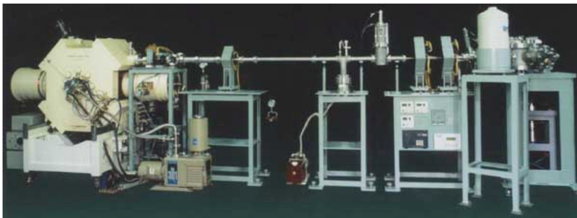
FIGURE 1. Whole view of the AVF cyclotron, the horizontal beam line and the vacuum chamber for PIXE measurements. The vertical beam line is not included in this photo.
