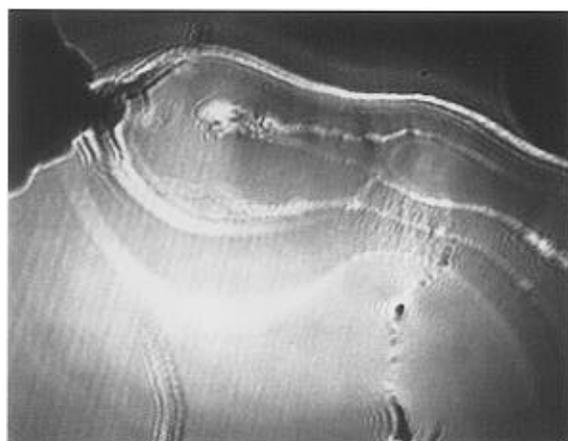
**Figure 7.** Multilayers of  $C_{60}$  at  $90 \text{ \AA}^2/\text{molecule}$  formed with a concentrated spreading solution.
