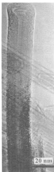
**Fig. 5.** HRTEM image from fibres found in the arc using BN-graphite mixtures. It is clear the appearance of inner core.
