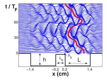
FIG. 6. Two cavities of width L=1.2 cm and depth h=0.5 cm, separated by a barrier of width  $L_b=0.4$  cm and depth  $h_b=0.092$  cm. The forcing amplitude is  $\Gamma=4.6$  with  $\Gamma_F\approx 5$  for the present geometry.
