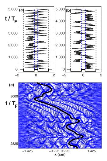
FIG. 7. Droplet tunneling at  $\Gamma=4.6$ . Cavity geometry as in Fig. 6: L=1.2 cm, h=0.5 cm,  $h_b=0.092$  cm. Observed Faraday threshold  $\Gamma_F\approx 5$ . (a)  $L_b=0.4$  cm with tunneling probability of 58%; (b)  $L_b=0.45$  cm with tunneling probability of 19%. Same initial conditions. (c) The wave field in an interval from panel (b) that includes a tunneling event.
