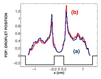
FIG. 11. Histograms of droplet position. Here,  $\Gamma=4.5$ ,  $\Gamma_F\approx5$ , L=1.2 cm,  $L_b=0.40$  cm, and depth  $h_b=0.092$  cm. (a) PDF for a single simulation with  $t\in[0,30\,000\,T_F]$ . (b) PDF for only 6 simulations with different initial droplet positions (3 in each cavity) and  $t\in[0,5000\,T_F]$ .
