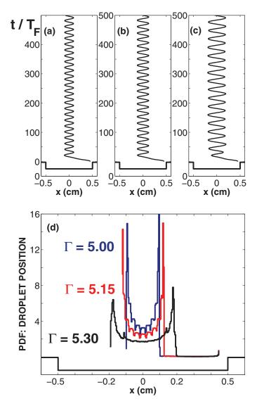
FIG. 9. Single-cavity oscillations: (a)  $\Gamma = 5.0$ ; (b)  $\Gamma = 5.15$ ; (c)  $\Gamma = 5.3$ . All with initial position at x = 0.45. (d) Histograms for periodic droplet motion reported in panels (a)–(c). Here  $\Gamma_F \approx 6.1$ .
