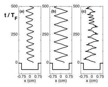
FIG. 4. A single cavity of length  $L=1.5\,\mathrm{cm}$  and depth  $h=0.5\,\mathrm{cm}$ . Three vertical accelerations are considered. (a)  $\Gamma=4.4$  yields an oscillatory droplet motion in the middle of the cavity. (b) When  $\Gamma=4.7$  the oscillatory droplet motion approaches the cavity's boundaries. (c) When  $\Gamma=5.2$ , the onset of chaotic droplet motion is apparent.
