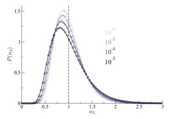
FIG. 3. (Color online) The distribution  $P(u_2)$  obtained from a numerical inversion of Eq. (13) for 3D systems. The curves from the dark to light correspond to  $\varepsilon = 10^{-3}$ ,  $10^{-4}$ ,  $10^{-5}$ , and  $10^{-6}$ . The symbols are results of numerical simulations of random walks for  $\varepsilon = 10^{-3}$  (circles),  $\varepsilon = 10^{-4}$  (squares),  $\varepsilon = 10^{-5}$  (triangles), and  $\varepsilon = 10^{-6}$  (diamonds).
