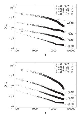
FIG. 7. Dislocation and chevron densities vs time for model II at different values of  $\varepsilon$ .
