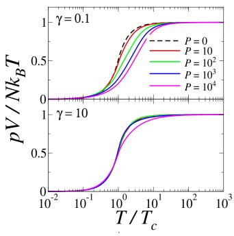
FIG. 5: (Color online) pV in  $Nk_BT$  units as a function of  $T/T_c$  for different values of the impenetrability parameter P. Upper panel is for  $a/\lambda_0 = 0.892$ ; lower panel is for  $a/\lambda_0 = 0.089$ .
