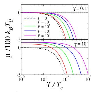
FIG. 4: (Color online) Chemical potential in  $k_B T_0$  units as a function of  $T/T_c$  for different values of the impenetrability parameter *P*. Upper panel is for  $a/\lambda_0 = 0.892$ ; lower panel is for  $a/\lambda_0 = 0.089$ .
