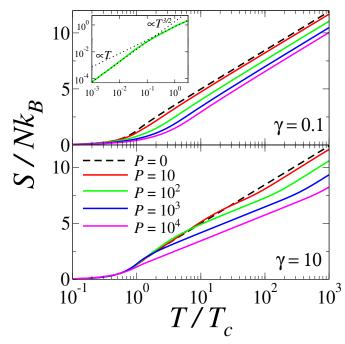
FIG. 8: (Color online) Entropy in  $Nk_B$  units as a function of  $T/T_c$ , for different values of the impenetrability parameter P. Upper panel is for  $a/\lambda_0 = 0.892$ ; lower one for  $a/\lambda_0 = 0.089$ . Inset in the upper panel shows the trapping effect as a change in the slope below the critical temperature.
