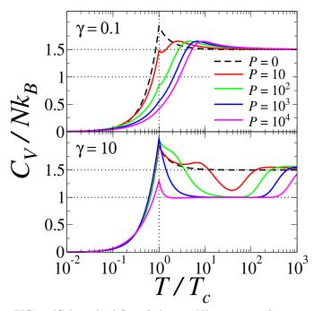
FIG. 7: (Color online) Specific heat in  $Nk_B$  units as a function of  $T/T_c$ , for different values of the impenetrability parameter P. Upper panel is for  $a/\lambda_0 = 0.892$ ; lower panel is for  $a/\lambda_0 =$ 0.089. Horizontal dotted lines denote the classical values for two- and three-dimensional IBG systems.
