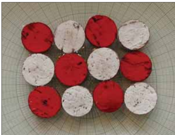
Fig. 3. Ionic model: (a) square lattice formed with six magnets with their dipole moment pointing upwards; (b) six with the opposite orientation.
