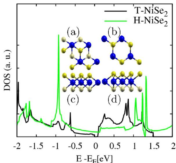
**Figure 1.** Electronic density of states without spin–orbit interactions and structure for the honeycomb (H) and centered honeycomb (T) lattices. Insets (a) and (b) are the T and H structures in the  $xy$  plane, respectively. Insets (c) and (d) display the T and H structures in the  $xz$  plane, respectively. We use slightly different colors to indicate which Se atoms are in the bottom layer (light yellow) and which are in the top layer (yellow). Ni atoms are in the middle layer (blue).
