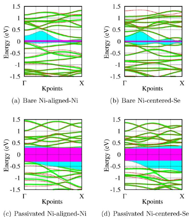
**Figure 6.** Electronic band structure for the corresponding two root armchair ribbons, both bare and H-passivated. The red and green lines correspond to calculations with and without spin-orbit interaction, respectively. The energy gaps are highlighted (see Table 1).
