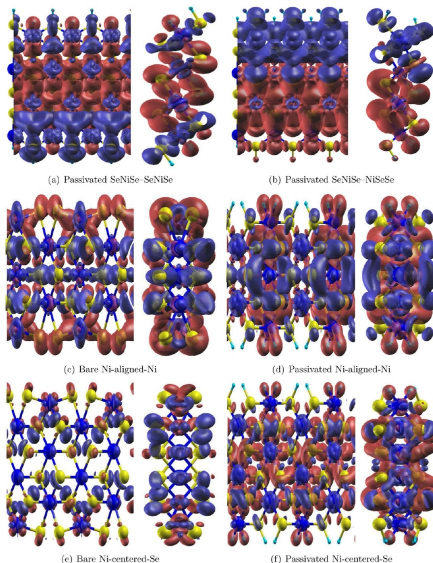
**Figure 10.** Charge density for the corresponding root zigzag and armchair semiconductor ribbons. Red and blue electronic clouds are maximum valence and minimum conduction bands, respectively. The isovalue for the surface is taken as 0.01 electron/Å<sup>3</sup>. Large (blue), medium (yellow), and small (aqua) circles are Ni, Se, and H atoms, respectively.
