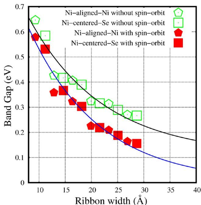
**Figure 7.** Band gaps of hydrogen passivated armchair ribbons as a function of width. The calculation without (green) and with (red) spin-orbit are included. The black (without) and blue (with spin-orbit interaction) solid lines are the corresponding fittings and are described within the text.
