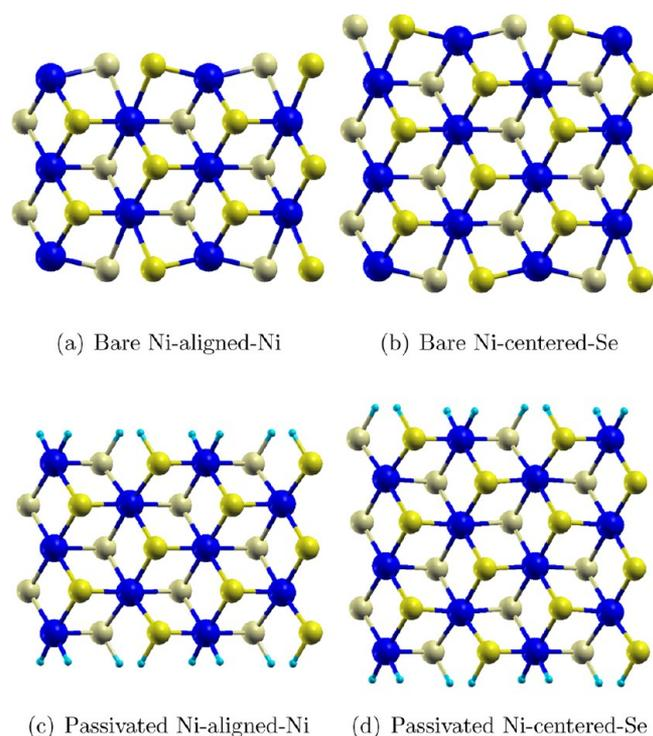
**Figure 4.** Graphical representation structure of the two root armchair ribbons, both bare and H-passivated. Large (blue), medium (yellow), and small (aqua) circles are Ni, Se, and H atoms, respectively.
