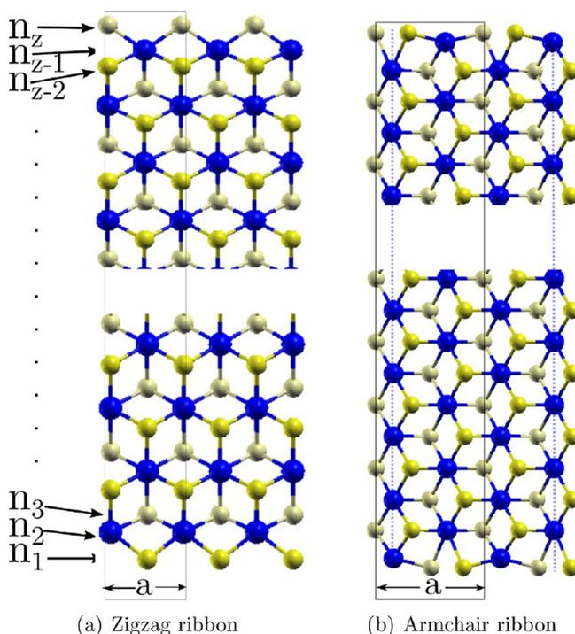
**Figure 2.** Nomenclature used to classify nanoribbons. Building blocks for the zigzag and armchair ribbons. For zigzag ribbons  $n_1, n_2, n_3, n_{z-2}, n_{z-1}$ , and  $n_z$  could be Se or Ni and  $z$  is the total number of rows in the nanoribbon. In the armchair case, the dotted line indicates if opposite edges present the Ni-aligned-Ni or Ni-centered-Se configurations. Large (blue) and small (yellow) circles represent Ni and Se atoms.
