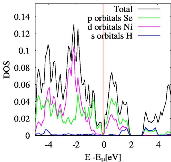
**Figure 9.** Total and partial density of states for the passivated zigzag SeNiSe–SeNiSe ribbon. The lowest valence band and the upper conduction bands are mainly Ni d-orbitals (magenta solid line) and Se p-orbitals (green solid line). Also, the H s-orbitals are presented (blue solid line).
