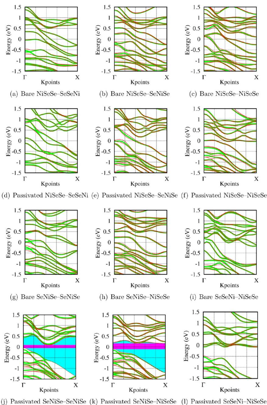
**Figure 5.** Electronic band structure for the corresponding six root zigzag ribbons, both bare and H-passivated. The red and green lines correspond to calculations with and without spin–orbit interaction, respectively. In the case of semiconductors (panels j and k), the energy gaps are highlighted (see Table 1).
