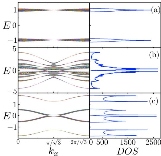
FIG. 7. (Color online) Band structure and density of states (DOS) of a ZGN for  $\phi = 0$ ,  $\lambda = 0.8$  using (a)  $\sigma = 1$ , (b)  $\sigma = (\sqrt{5} - 1)/2$ , and (c)  $\sigma = 1/4$ . The same conditions as in Fig. 6 were used. Note the big gap opened at the Fermi level in (a); in (b) the band structure is fragmented and hence the DOS has a lot of spikes, and in (c) the DOS is similar to that of linear chains weakly interacting.
