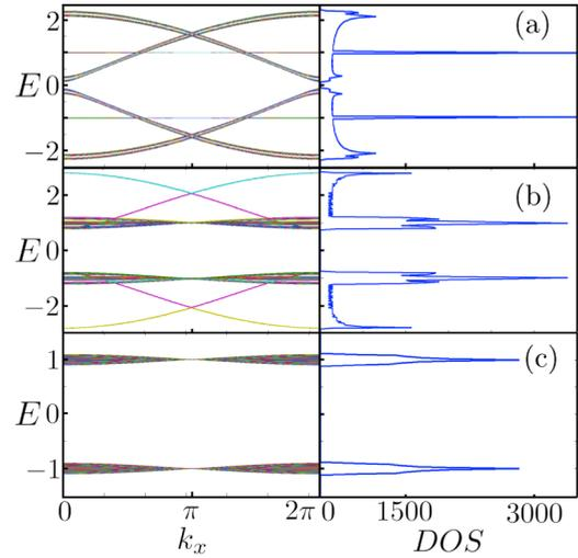
FIG. 4. (Color online) Band structure and density of states (DOS) of an AGN for  $\phi = 0$  and  $\lambda = 0.8$  using (a)  $\sigma = 0.6/\sqrt{3}$ , (b)  $\sigma = 0.8/\sqrt{3}$ , and (c)  $\sigma = 1/\sqrt{3}$  for a system with 200 atoms. Cyclic boundary conditions were used.
