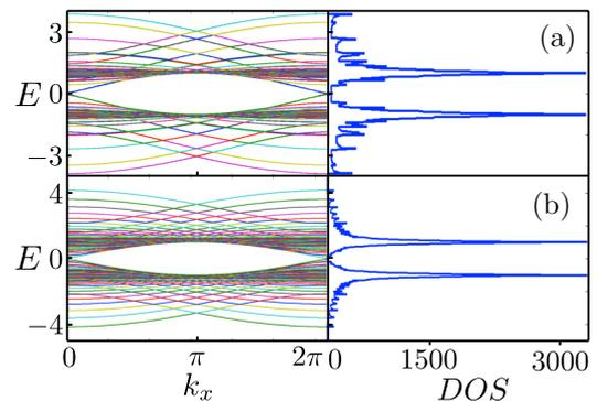
FIG. 5. (Color online) Band structure and DOS for an AGN using (a)  $\sigma = 4\sqrt{5}/3$  and (b)  $\sigma = 0.4\sqrt{7}/3$  for  $\alpha = 0.4$  and the same conditions as in Fig. 4. Note that there are two partially flat bands at  $E = \pm 1$  and that the DOS is spiky.
