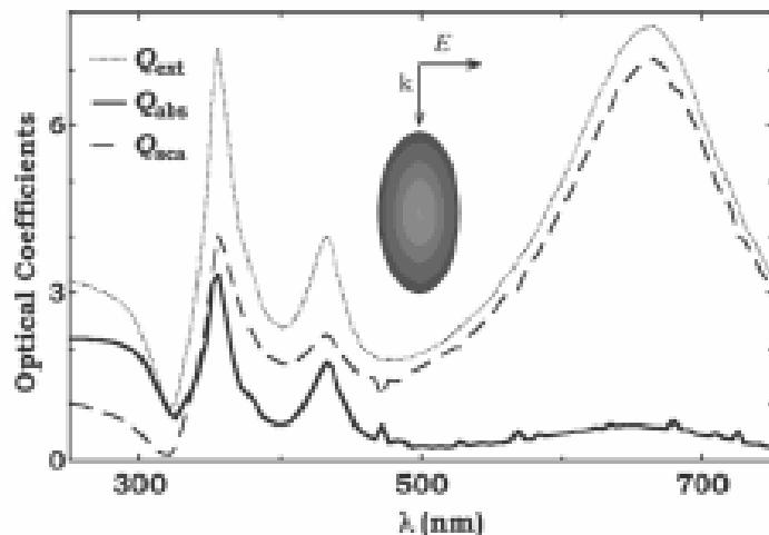
Figure 3. Optical coefficients for a silver nanospheroid for an electric field polarized along the minor axis.
