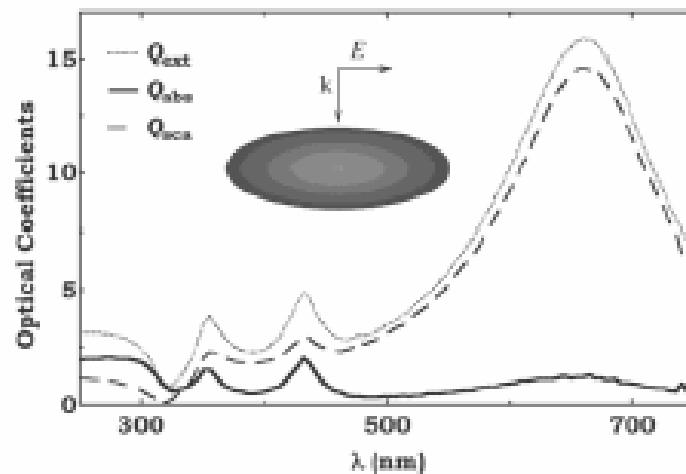
Figure 4. Optical coefficients for a silver nanospheroid for an electric field polarized along the major axis.
