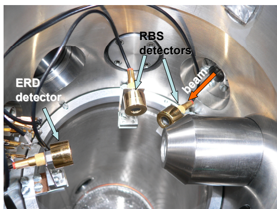
FIGURE 2. Particle detector arrangement for simultaneous RBS (135° IBM- and 165° Cornell-geometry) and ERDA (30° IBM-geometry) measurement.
